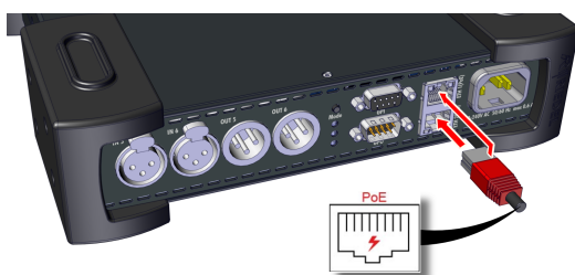
figure 13: powering via PoE
